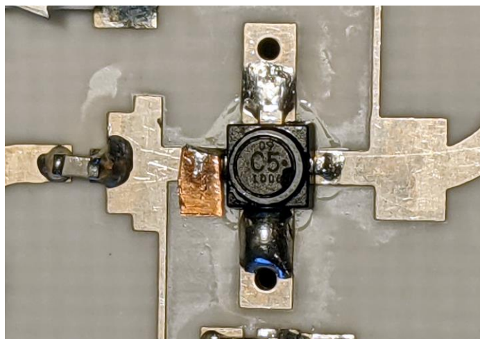
Figure 8 Tuning flake on Q8 drain
