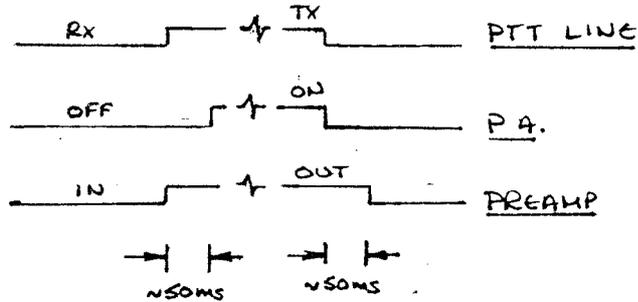
A wide variety of inputs may be used to control the sequencer. Many transceivers provide either a positive dc level or an externally accessible relay contact which makes to ground when on transmit. Other transceivers output a positive dc level via the antenna socket: this may be present either on transmit or receive. A few transceivers have no control output at all.
