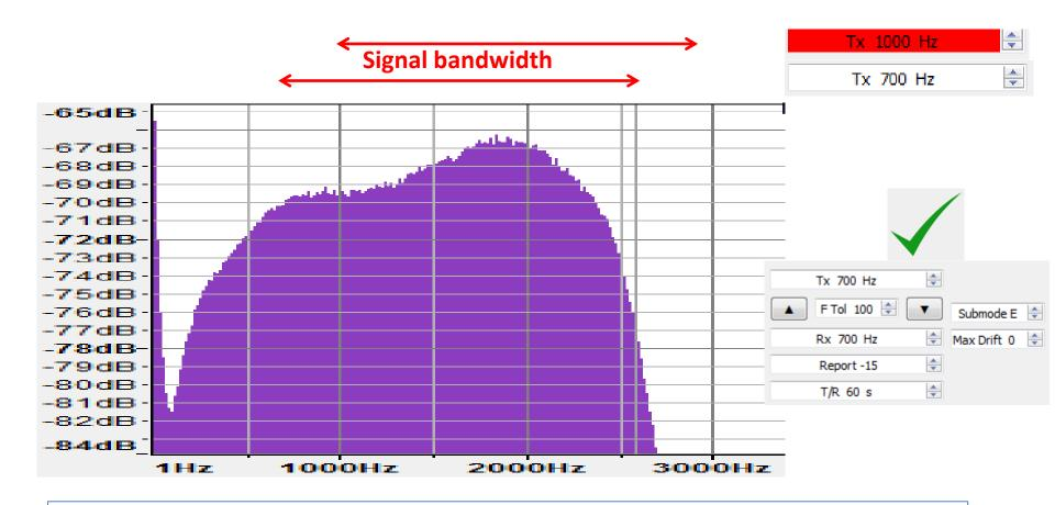
Limitations in the upper edge of the passband can sometimes be compensated, for by driving one or more stages of the RF stages in the TX chain into compression.
