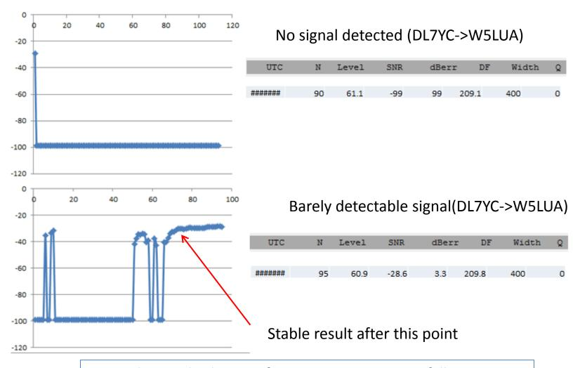
Note: This method outperforms Linear Avg waterfall spectrum for detection of very weak signals with wide spreading.
