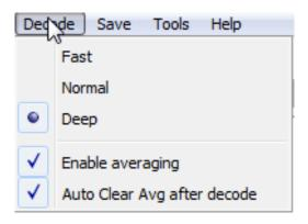
Fast, Normal and Deep options are available. Fast will decode most signals; for very weak signals. Deep may be needed, but the decoding process will generally take longer.
