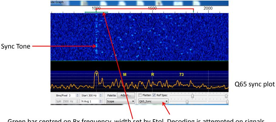
Green bar centred on Rx frequency, width set by Ftol. Decoding is attempted on signals within width of green bar. If signal is too weak to see on waterfall, and you are not sure of frequency, then a wide Ftol should be used (at the expense of decode time and possible loss of sensitivity). In most cases start with 100Hz, but experimenting may prove useful in some cases.
