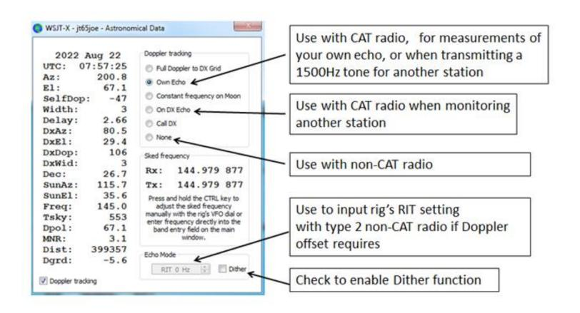
Note: A 'type 2 non-CAT radio' has ability to set RIT by a known, precise, amount to bring received signal close to 1500Hz.
