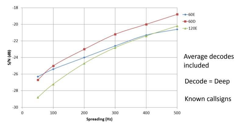
This graph allows optimum choice of sub-mode for different spreading conditions. For example, at 100Hz spreading 120E would be the best mode, followed by 60E, which is slightly better than 60D. At 500Hz, 60E is slightly better than 120E, and 60D would perform worst.
