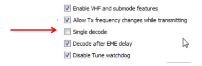
Decoding the whole passband increases decode time, and needs signals to have higher S/N, compared to single decoding. <u>Multi decoding only works if Max</u> Drift is set to 0.
