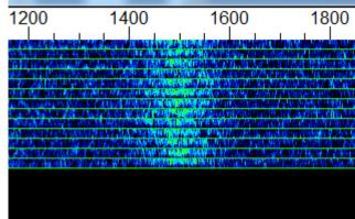
System: 2.4m dish, 70W at feed. Spread = 221Hz
