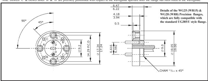
A Holes 4 off - 4.40 UNC-2B. C'bore 3.56 dia x 1.6 dia deep from flange face
