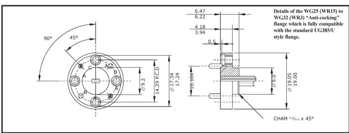
A Holes 4 off - Drill 4.40 UNC-2B. C'bore 3.56 dia x 1.6 dia deep from flange face
