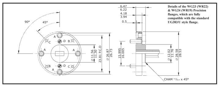
A Holes 4 off - 4.40 UNC-2B. C'bore 3.56 dia x 1.6 deep from flange face
