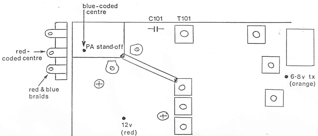
17. Lead the cables neatly around the SLNA 145sb ensuring that none of the cables or leads run across the board, and then replace the antenna screening tube in its previous position.
