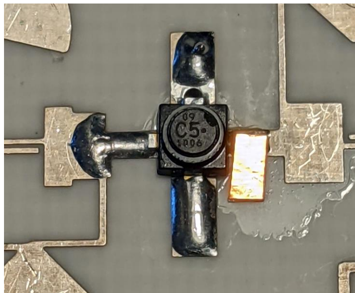
Figure 9 Tuning flake on Q9 gate
