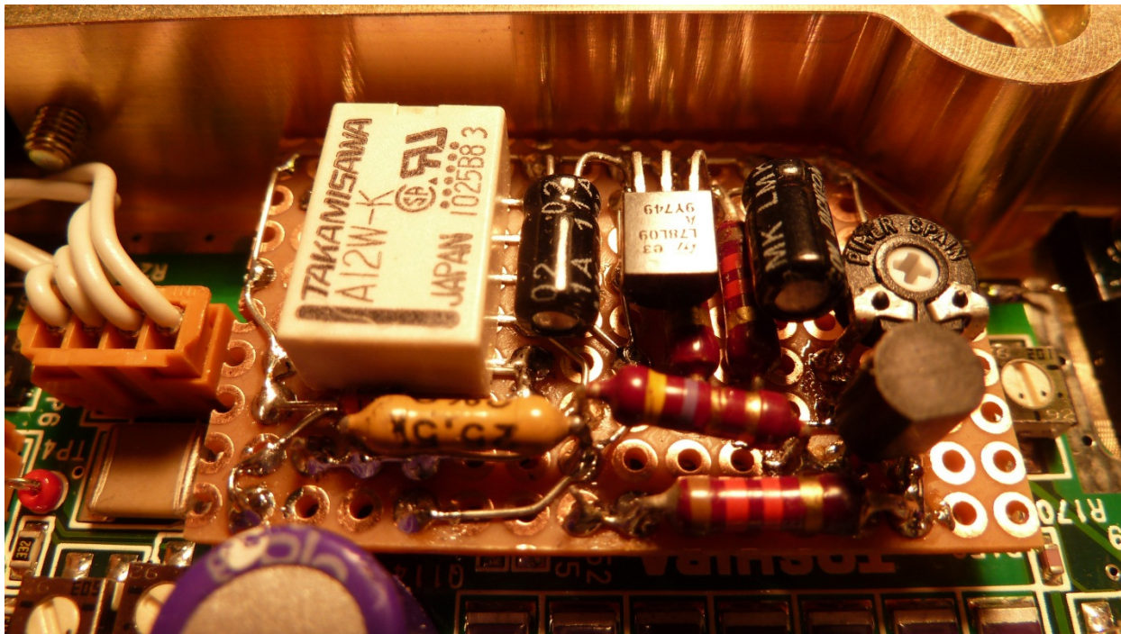
Figure 10: Macro picture of the new PSU board in place
