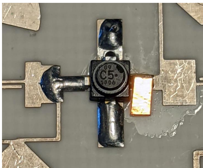
Figure 9 Tuning flake on Q9 gate
