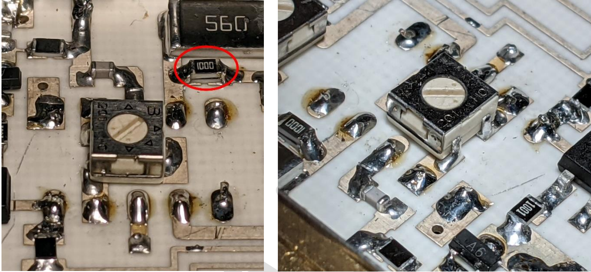
Figure 6 Location of R3 variable between the legs of the relay. Second view is from top left of the first. Red ring shows low power IF modification with 100R fitted over R8
