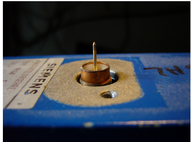
BETTER: End of the coaxial Helix system - The WG must fit very tight to the outer dia
